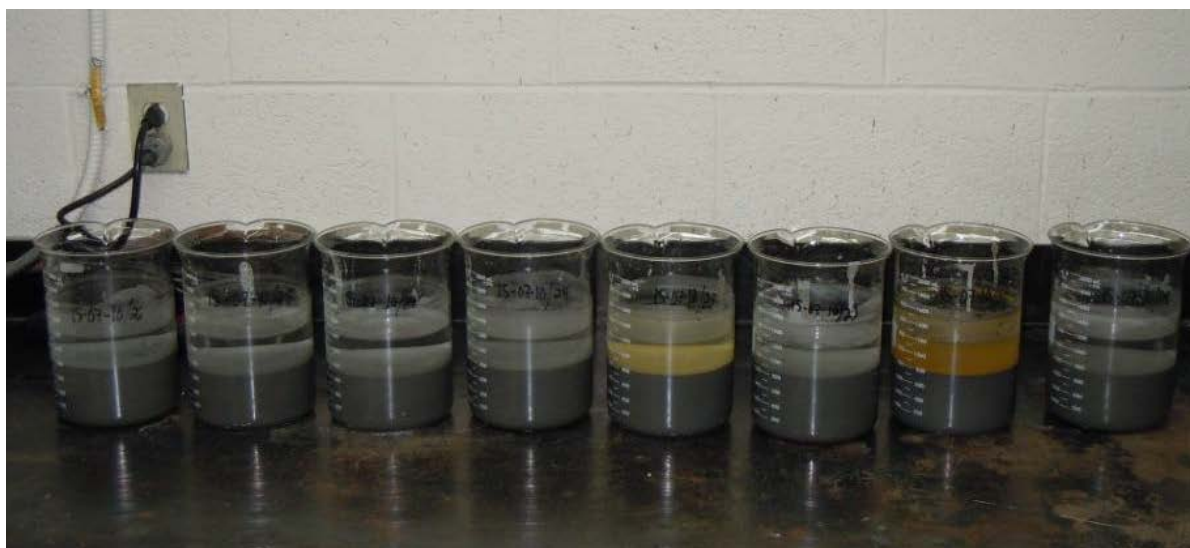
Figure 3: Arsenic Treatment Tests after Settling Overnight
