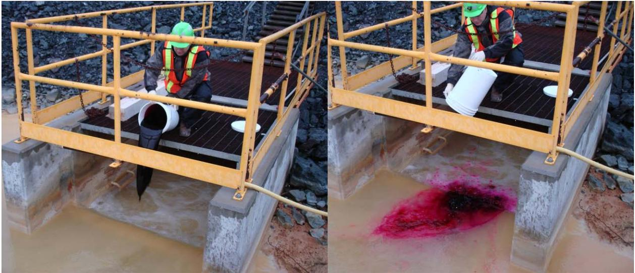
**Figure 2: Injection of Tracer into Pond 1B Feed Culvert**
