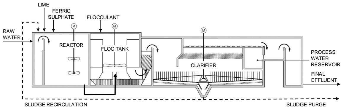
**Figure 3** Process system at the Bloom Lake WTP
