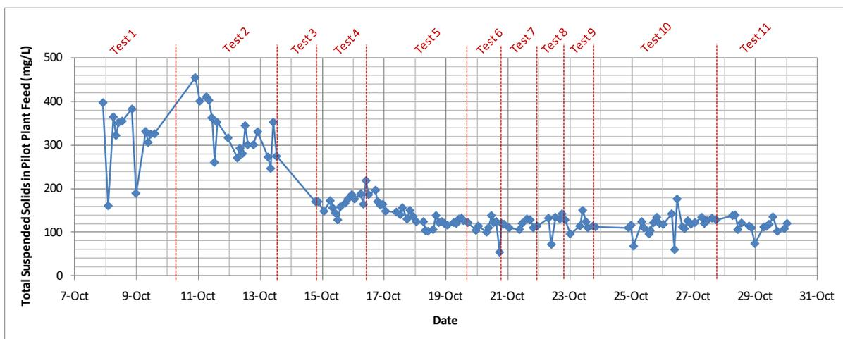
**Figure 2** Raw water total suspended solids during piloting
