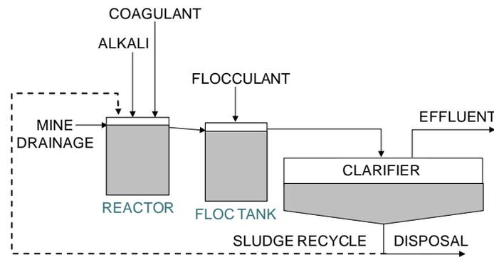
**Figure 1** Process applied during piloting
