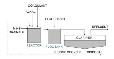
Figure 1 Process applied during piloting
